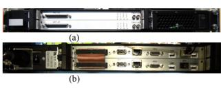
Figure 5:(a) CPSCI AO32 frontend. (b)CPSCI AO32 backend. 32 channels AO is extend to 64 channels AO by RTM-AO16 bus.
