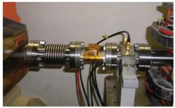
Figure 4: Typical installation for RadFET sensors.
