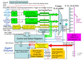
Figure 8: Functional block diagram of the corrector power supply controller (CPSC) module.
