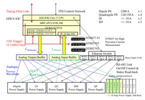
Figure 1: Control infrastructure of TPS booster ring power supplies.
