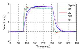
Figure 2: Step response of dipole and four quadrupole power supplies. Dipole and QF had slower response due to larger magnet loading.
