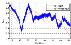
Figure 5: The inferred input (red) from output (blue).
