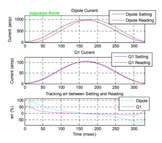
Figure 3: Ramping waveform of Dipole and Q1. Different phase delay will cause different tracking err between setting and reading.
