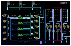
Figure 4: Chilled Water System in U2.
