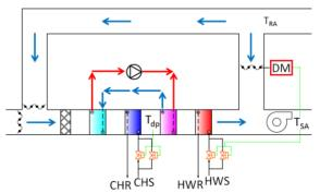
Figure 2: Control Diagram of High Precision Temperature Control System.
