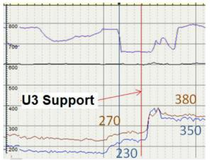
Figure 5: Power Consumption During U3 Chillers Supply Chilled Water.
