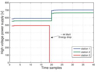
Figure 5: The high voltage value of the three klystrons at the SwissFEL injector test facility.
