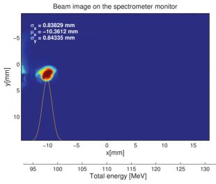
Figure 3: The electron beam image captured at the spectrometer camera. The x-position of the beam is used to estimate the beam energy.
