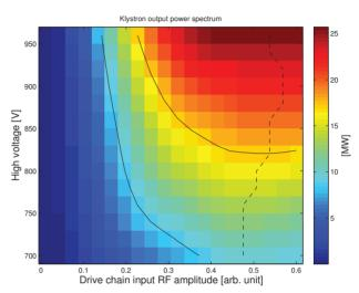
Figure 1: The klystron output power versus the RF input amplitude and the high voltage power supply setting. The curves (in black) denote the contours of constant output power. The dashed line indicates the saturating power. The klystron operating point should fall in the left side of the dashed line to avoid over-saturation.
