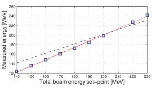
Figure 2: The total measured beam energy versus the reference (setpoint) energy. The dashed-line, which simply plots the equation y = x, represents the ideal open-loop response.
