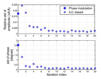
Figure 4: The standard deviation of the BOC output RF amplitude and phase waveforms over the flat-topped region.
