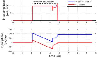
Figure 3: The klystron input amplitude and phase waveforms for phase modulation regime (in blue), and the ILC-based method (in red) after 20 iterations.
