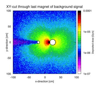
Figure 4: Beam pipe shields the cross-talk from the second beam. Detector position in the vertical plane at y = 0 cm.
