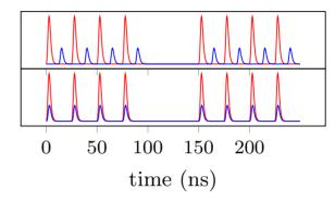
Figure 2: Example for loss signals of unmatched (top) and matched (bottom) beam losses of both beams, primary beam in red.
