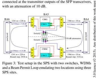
Figure 3: Test setup in the SPS with two switches, WDMs and a Beam Permit Loop emulating two locations using three SPS sites.
