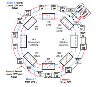
Figure 1: LHC beam permit loops.
