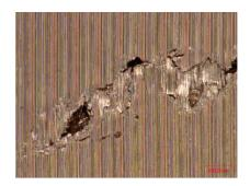
Figure 7: Micro-Cavity at z=85 cm in Target 3. The area is located on the beam axis with a surface of  $\sim 1.5$  mm<sup>2</sup>.
