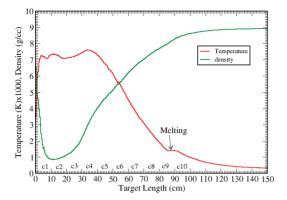
Figure 2: Simulation Results:  $\varrho$  and T vs target axis at t = 7850 ns for target 3, after irradiation with 144 bunches [3].
