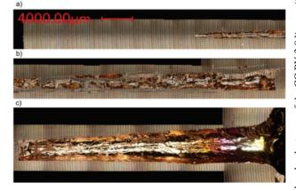
Figure 5: Target 3, Cylinder 1. Microscopic analysis of the hole generated by the beam. a) first, b) second and c) last third of the cylinder.
