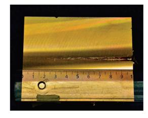
Figure 4: Surface picture of Cylinder 1 of target 3 after cutting it longitudinally. In the first 2.3 cm micro cavities are observed, further downstream a cone shaped hole is clearly visible.
