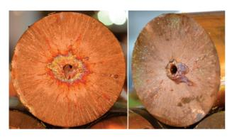
Figure 3: Front (left) and back (right) faces of the third cylinder of target 3. Re-solidified copper splashes and the hole generated by the beam is visible.
