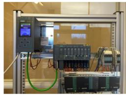
Figure 4: Prototype for magnet powering interlocks.
