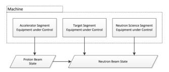
Figure 1: Simplified representation of the "machine". Equipment under control from the accelerator segment controls the proton beam state. The neutron beam state is controlled by the Target and Neutron Science Segment EUC and is influenced by the proton beam.
