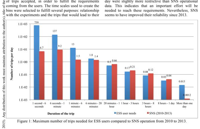
Figure 1: Maximum number of trips needed for ESS users compared to SNS operation from 2010 to 2013.
