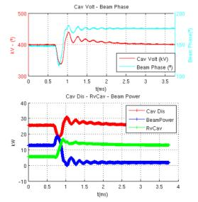
Figure 2: Response of active cavities after RF failure and partial beam loss.
