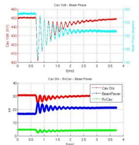
Figure 1: Response of active cavities after RF failure and beam survival.
