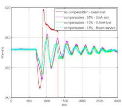
Figure 4: Comparison of different Feed-Forward Settings after a forced RF trip.
