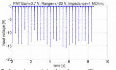
Figure 7: Injection-to-injection losses. Time constant is about 13 ms at 1 M $\Omega$  input impedance.
