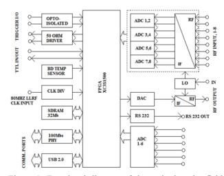
Figure 1: Functional diagram of the revised cavity field controller.
