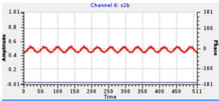
Figure 4: CFC scope trace in EPICS showing phase modulated beam pickup signal at synchrotron frequency.
