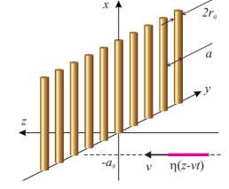
Figure 1: Bunch passing by the edge of a a grid structure.
