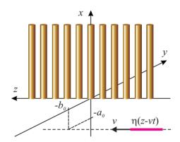
Figure 2: Bunch moving along the edge of a grid structure
