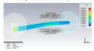
Figure 11: Beam dynamics simulation in CST.
