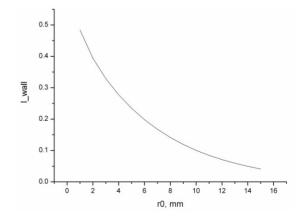
Figure 7: Image current on the wall.
