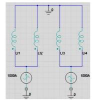
Figure 4: Simplified equivalent electrical circuit of the magnet.
