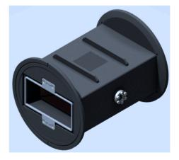
Figure 2: 3D drawing of the beam position monitor.
