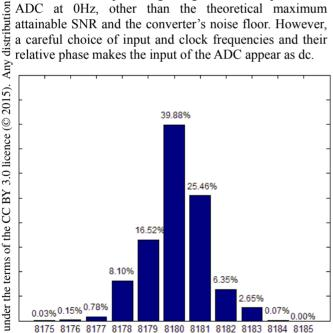
Figure 2: Histogram of sampling system under test with DC input applied. The x-axis represents the ADC output code in LSBs, and the height of the barrels is the percent may hit count for each code in a run of 16384 sample points. The mean of the distribution is 8180 LSBs, indicating an offset of approximately 12 LSBs.
