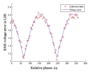
Figure 3:  $\sigma_V$  vs.  $\Delta \phi$  at 100MSps clock rate with 2ps jitter, 100MHz coherent input: the  $\sigma_V$  due to jitter amounts to 2.26LSB.
