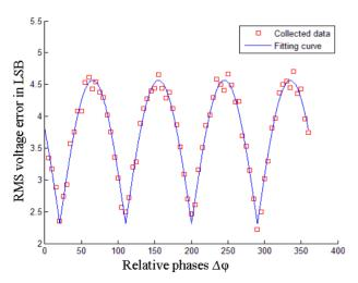
Figure 4:  $\sigma_V$  vs.  $\Delta \phi$  at 100MSps clock rate with 2ps jitter, 200MHz coherent input: the  $\sigma_V$  due to jitter amounts to 4.61LSB.
