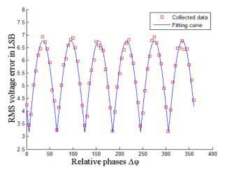
Figure 5:  $\sigma_V$  vs.  $\Delta \phi$  at 100MSps clock rate with 2ps jitter, 300MHz coherent input: the  $\sigma_V$  due to jitter amounts to 6.83LSB.
