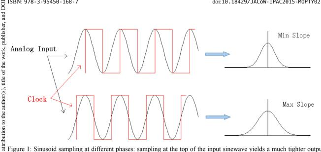
Figure 1: Sinusoid sampling at different phases: sampling at the top of the input sinewave yields a much tighter output code distribution than sampling the input at its maximum slope (zero-crossing).
