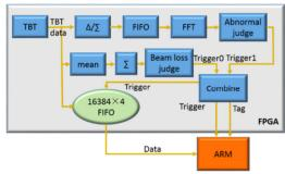
Figure 3: Function diagram.
