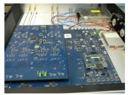
Figure 2: DBPM processor.
