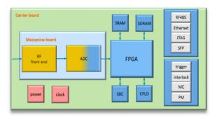
Figure 1: DBPM processor architecture.
