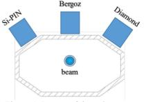
Figure 4: Layout of three detectors.
