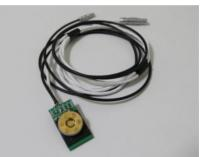
Figure 3: Prototype of CVD diamond BLM detector.
