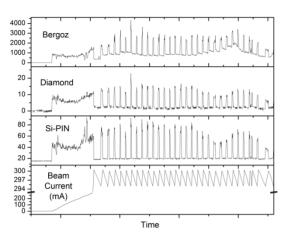
Figure 5: Comparison of Diamond, Si-PIN and Bergoz detector.
