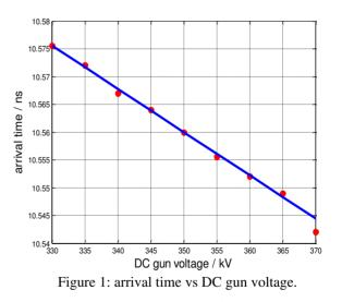
Here, the red dot is the result of ASTRA simulation, while the blue line is theoretical result obtained from Equ. (1), and the same setting is used in following figures.
