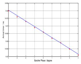
Figure 4: arrival time versus buncher phase.
