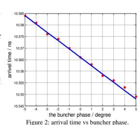
From Fig. 1, Fig. 2 we can see that the relation between arrival time jitter and DC voltage or buncher phase fits quite well with the theoretical line.
