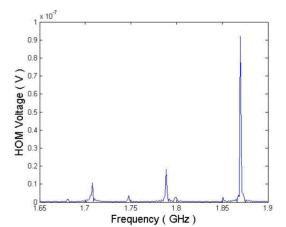
Figure 2: Simulated HOM spectrum, which is excited by a train of bunches at the repetition rate of 81.25MHz.
