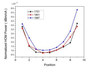
Figure 4: Normalized power of IF peaks at various beam offset in the SRF cavity. Position number is used as the horizontal coordinate instead of the beam positon since the absolute position has not been calibrated.
