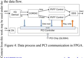
Figure 4: Data process and PCI communication in FPGA.
