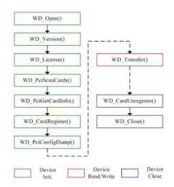
Figure 5: Software flow of data transfer in WinDriver.
