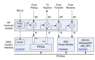
Figure 2: Structure of one LLRF control unit.
