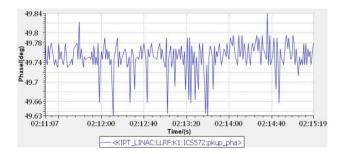
Figure 6: Phase detection by ICS572F board.
