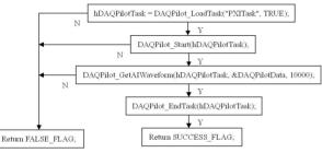
Figure 3: DAQ flow of PXI9846.
