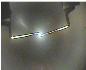
Figure 3: Polarimeter target deformation at store due to electrostatic interaction with proton beam. The electric fields are stronger due to smaller beam size and higher beam current. The whole chamber is lighted.
