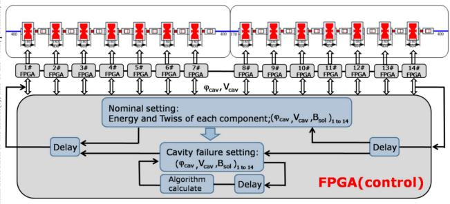
Figure 1: Diagram of the hardware compensation in C-ADS.
