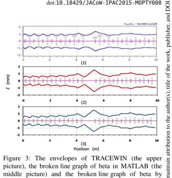
Figure 3: The envelopes of TRACEWIN (the upper picture), the broken line graph of beta in MATLAB (the middle picture) and the broken line graph of beta by hardware simulation (the down picture).
