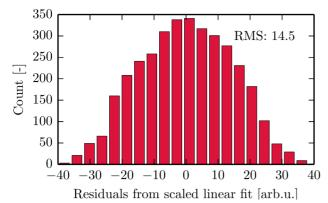
Figure 5: Residuals of the linear fit from Fig. 4, scaled so that the average WFM and BPM measurements give the same value. The RMS of the residuals of 14.5 then gives a merit for the precision.
