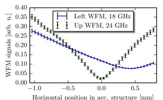
Figure 2: A scan over horizontal positions. The 'Left' signal filtered at 18 GHz and the 'Up' signal filtered at 24 GHz are shown.
