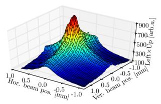
Figure 6: A scan of the WFM signals in both planes. The 'Left' and 'Up' signals at 24 GHz are multiplied, which gives a peak at the position of the center of the structure.
