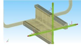
Figure 1: The internal geometry of a TD26 structure except for the first coupling cell. The WFM waveguides are shown in green and the pickup antennas in red.
