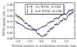
Figure 3: A scan over vertical positions. The 'Up' signal filtered at 18 GHz and the 'Left' signal filtered at 24 GHz are shown.
