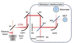
Figure 2: Schematic diagram of the Michelson interferometer. M: aluminium mirror, OAP: off-axis parabolic mirror, BS: beam splitter.
