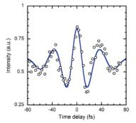
Figure 4: Interferogram of CTR and fitting curve using Eq. 6.
