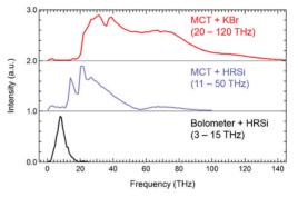
Figure 3: Frequency spectra of IRS detected in case of different combinations of infrared detectors with beam splitters.
