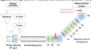
Figure 1: Schematic diagram of a laser photocathode RF electron gun linac and a magnetic bunch compressor. Q: quadrupole magnet; B: bending magnet; S: sextupole magnet.
