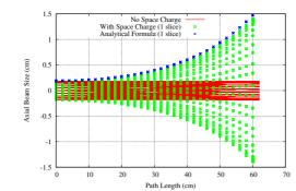
Figure 1: Axial beam envelope in a drift. The analytical formula (8) in blue shows that the space charge kick is applied correctly.
