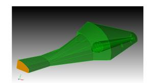
Figure 1: CUBIT quarter model of the horizontal separator.
