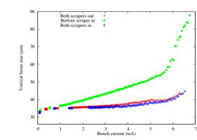
Figure 8: Vertical beam size vs current, with different scraper configurations. There is a strong beam size blowup when only the bottom scraper is inserted.
