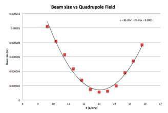
Figure 2: Beam size as a function of quadrupole field strength in the horizontal plane at ASTA using quadrupole Q112 on a YAG imaging screen at the imaging station X120.
