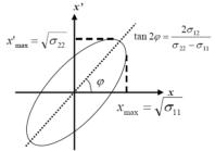
Figure 1: Beam ellipse with physical interpretation of the physical components [1].
