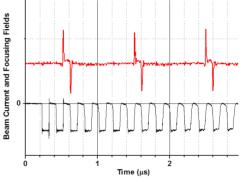
Figure 1: Synchronization between the barrier bucket fields (red) and beam current (black) from the wall-current monitor in the ring.
