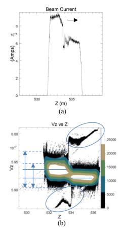
Figure 4a-b: (a) – Beam current at turn 45, at a compression rate of 0.5 ns/turn. (b) – Longitudinal ( $v_z$ -z) phase-space at the same compression rate.
