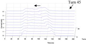
Figure 2: Beam current with compression at a rate of 0.5 ns/turn.
