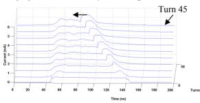
Figure 3: Beam current with compression at a rate of 1.0 ns/turn
