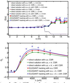
Figure 3: (Top) CSR gain functions G(s), where the dashed lines are for  $\lambda = 0.5$  mm and solid lines for  $\lambda = 3$ mm. (Bottom) gain spectra  $G_{\ell}(\lambda)$ . Here in ELEGANT simulation the initial density modulations are all set 1 %.
