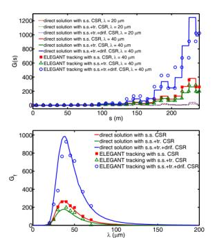
Figure 1: (Top) gain functions G(s) as a function of s, where the dashed lines are for  $\lambda = 20$  mm and solid lines for  $\lambda = 40$  mm. (Bottom) gain spectra  $G_f(\lambda)$  as a function of modulation wavelength. In ELEGANT simulation, the initial density modulation is set 0.05 % for steady-state (s.s.) case; 0.06 % for s.s. and entrance transient (tr.) case; 0.01-0.04 % for s.s., tr. and exit transient (drif.) case.
