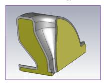
Figure 2: "Mirror" walls in 1/8 cavity model.
