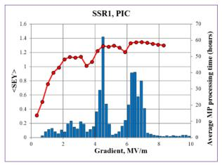
Figure 4: Simulated MP barriers and average processing time required to get through the barriers.
