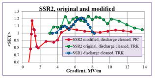
Figure 7: Reduced <SEY> in modified SSR2 cavity compared to the original design and SSR1.
