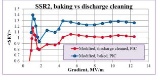
Figure 8: The simulations of MP in SSR2 with different surface treatment.
