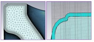
Figure 1: Tetrahedrahedral mesh used in eigenmode solver and hexahedral mesh used for tracking.
