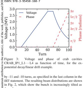
Voltage and phase of crab cavities Figure 3: CRAB IP1 L1···L4 as function of time, for the exponential decay/linear drift example.
