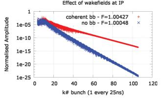
Figure 4: Normalised actions of the bunches at the IP. Only the bunch with action 1 carries an initial misalignment. All the other bunches are excited by LRW. The bunches contains  $4 \times 10^9$  electrons.
