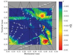
(d) Vertical scan from top to bottom conducted after the realignment. Beam loss along the resonance  $-q_x + 3q_y = 0$  in the bottom right corner corresponds to an interpolation artifact.
