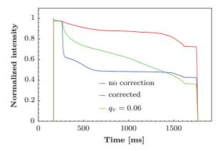
Figure 4: Influence of orbit correction on beam loss. For the blue and red curves the vertical tune was programmed to 6.10. With an active correction the vertical tune could be programmed closer to the integer resonance (green curve), which was impossible without correction.
