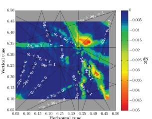
(b) Vertical scan from top to bottom conducted before the realignment. Beam loss along the vertical line  $Q_x = 6.35$  corresponds to an interpolation artifact.
