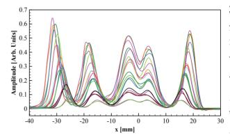
Figure 1: Example of islands profiles measured by a wire scanner and for different intensity [3]. The displacement of the islands centers with intensity is apparent.
