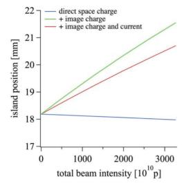
Figure 5: Island position with total beam intensity. Direct space charge produces a negative tune shift and the island moves inward with intensity. The image charge only gives the positive tune shift and the island moves outward. The image current partially cancels the tune shift and the gradient is less than the case with the image charge only. Beam momentum is 14 GeV/c, half vacuum chamber height is is h=35 mm, and half magnet pole face height is g=50 mm.
