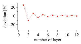
Figure 4: Deviation of the fixed point position with different numbers of the image charge/current layers on one side. In this test, the total number of particles is  $2.0 \times 10^{13}$ , the beam momentum is 14 GeV/c, the half vacuum chamber height is h=35 mm, and the half magnet pole face height is g=50 mm.
