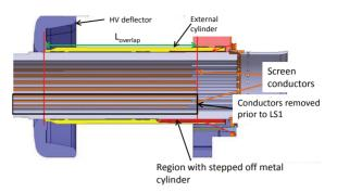
Figure 1: Cross-section of the beam screen of the MKI. Conductors circled in red weren't in place prior to longshutdown 1.
