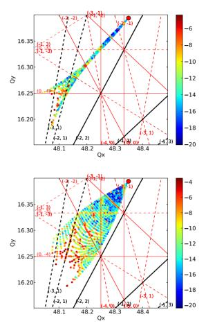
Figure 5: Top: Frequency map for the perfect aligned lattice with a linear hard-edge wiggler. Bottom: Frequency map including a thin octupole per wiggler period.
