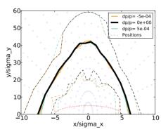
Figure 4: On and off-momentum DA for the lattice fed with errors at the obtained tolerances.
