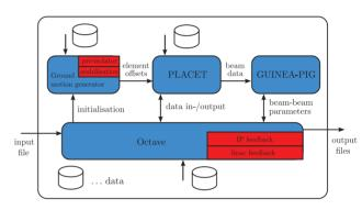
Figure 1: Internal structure of LinSim, where scripts (written in Tcl and Octave) interface the simulation codes PLACET, a ground motion generator, and GUINEA-PIG. An input file is used to control the simulations that use additional data such as lattice files and created standardised output files.
