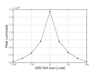
Figure 3: Peak luminosity in  $cm^{-2}s^{-1}$  versus QD0 roll.
