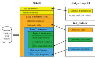
Figure 2: Structure of a simulation with LinSim (entry point is run.tcl), which used external data and is controlled via two test file, e.g. test\_settings.tcl and test\_code.m. Code from test files is linked into four different parts of the execution, which increases the flexibility significantly.
