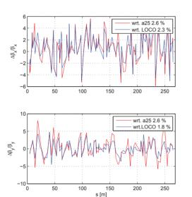
Figure 4: Beta beat measurement at the quadrupoles respect to the bare model (red lines) and respect to the model reconstructed by LOCO (blue lines). The upper plot shows the horizontal values while the lower one shows the vertical ones.
