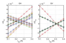
Figure 3: Tune difference with respect to the nominal as a function of the recovery current. Each family is represented in a different color. Horizontally focusing magnet families are shown in the left hand side plot while the vertical focusing ones are in the right hand side plot. The horizontal tune is represented by positive slope lines in the left hand side plot and by negative slope lines in the right hand side plot, the other way around for the vertical tune.
