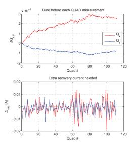
Figure 5: The upper plot shows the tune change after each magnet measurement and having applied the corresponding recovery current. The lower plot shows the corresponding additional recovery current to compensate each tune change.
