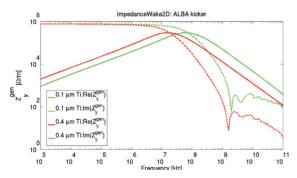
the CC BY 3.0 licence (© 2015). Any distribution of this Figure 4: Vertical generalized impedance of the pinger magnet. In red, the Ti thickness assumed is 0.4  $\mu$ m. In green, a thinner coating is considered of 0.1  $\mu$ m.
