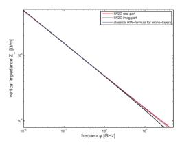
Figure 1: wall impedance of std vacuum chamber. At high frequency the imaginary part is smaller than both the real part and the one given by the classical RW-formula for monolayers.
