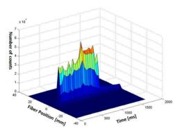
Figure 2: SFH acquisition (20 Hz acquisition rate, 20 ms shutter time) of a 65 MeV/u Protons spill (about 10<sup>8</sup> particles) on the horizontal plane.
