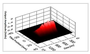
Figure 5: SFP acquisition (300 Hz acquisition rate, 2.8 ms integration time) of one 111 MeV/u Protons spill (about 10<sup>8</sup> particles) on the horizontal plane.
