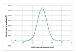
Figure 7: Beam horizontal profile reconstruction performed with the WD by using one vertical fiber.
