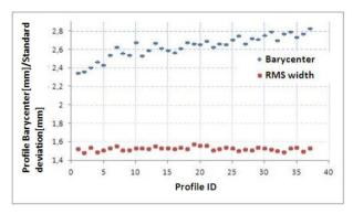
Figure 4: Computed barycenter and standard deviation values for 37 horizontal beam profiles acquired by the QPM during one spill extraction.
