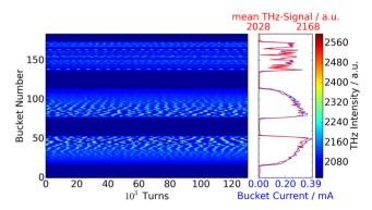
Figure 1: The peak-intensity of the THz pulses of all 184 RF-buckets is displayed over 130 thousand consecutive turns and shows strong fluctuations caused by bursting. A typical measurement takes one second and contains 2.7 million turns. The graph to the right shows the filling pattern.
