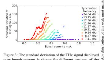
Figure 3: The standard deviation of the THz signal displayed over bunch current is shown for different settings of the magnet optics (with constant RF-voltage), which result in different synchrotron frequencies indicated by color [7].
