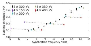
Figure 4: The bursting threshold for a combined scan is shown over the synchrotron frequency. The error bars include the error of the algorithm for the automated threshold detection, the bunch current measurement as well as the expected spread of the threshold due to multi-bunch effects.
