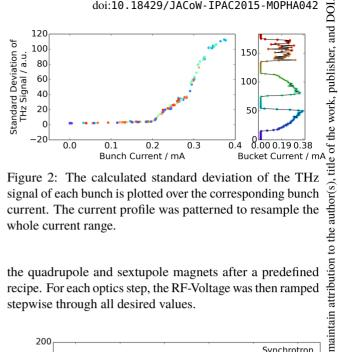
Figure 2: The calculated standard deviation of the THz signal of each bunch is plotted over the corresponding bunch current. The current profile was patterned to resample the whole current range.
