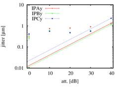
Figure 2: Jitter measurement for the 3 BPMs. The dotted lines are extrapolation of noise at 40 dB.
