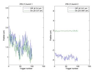
Figure 3: Effect on second bunch position (right) from first bunch position (left) feedback.
