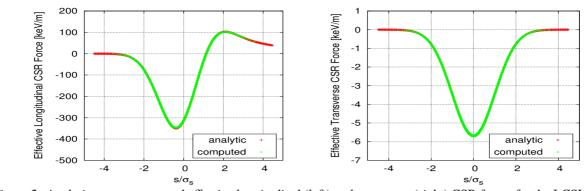
Figure 2: Analytic versus computed effective longitudinal (left) and transverse (right) CSR forces for the LCSL bend [3]: N = 1024000 particles on a 64 × 64 grid, bend radius  $R_0 = 25.13$  m,  $\theta_b = 11.4^\circ$ , longitudinal rms beam size  $\sigma_s = 50 \mu$ m, emittance  $\epsilon = 1$  nm, and total beam charge of Q = 1 nC.
