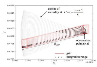
Figure 1: Integration for the retarded potential quadrature in Eq. (4) for a typical grid point. The black lines represent the limits of integration in  $\theta'$ .
