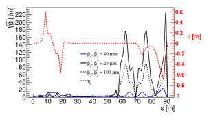
Figure 1:  $\beta$  functions and dispersion along the ATF2 beam line in case of nominal  $\beta_y^*$  and ultra-low  $\beta_y^*$  optics.  $\beta_x^*$  is increased by a factor 10 to minimize horizontal to vertical coupling.
